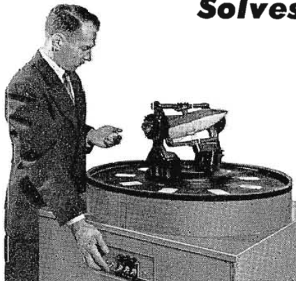
Scale model used to simulate the behavior of a guided missile under actual flight conditions.
