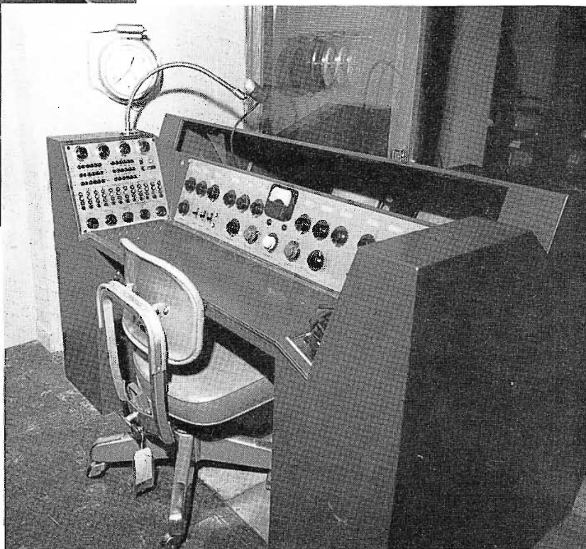
FIG. 5. The NBC Custom TV-Audio console shown installed at El Capitan theatre studio.
